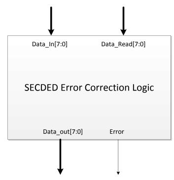
The Data\_Out[7:0] output should return the correct data when there is no error, and when there is a correctable single-bit error (so your design must correct the corrupted bit).
