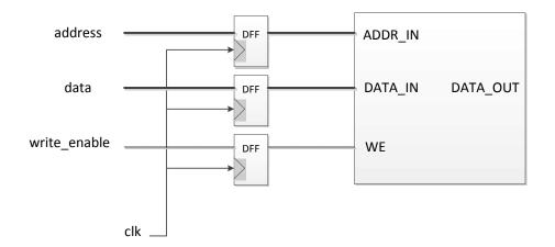
Answer: Because the WE signal is asserted immediately after the address and data become valid, and unasserted immediately after the address and data become invalid. It violates both the setup and hold time constraints of the memory.
